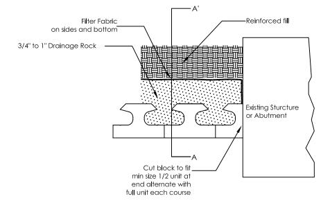
Provide for drainage away from wall. (i.e. Drainage Swale or impermeable soils.) 3/4" to 1" Drainage Rock Existing Structure or Abutment Filter Fabric on sides and top <u>A-A'</u> Drain Tile
