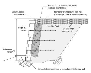
\*Minimum 6" embedment or 10% of wall height. Embedment increases with increased wall heights, sloping fills in front and behind wall or poor foundation soils. Contact professional geotechnical engineer for guidance.
